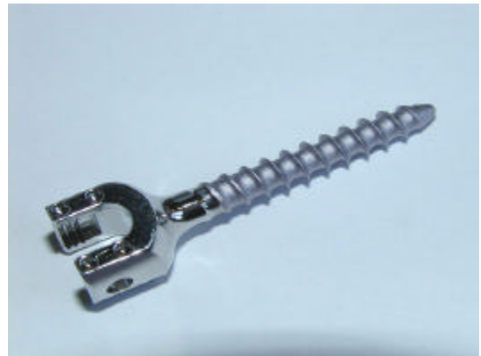
Examples of tantalum coated parts: Nozzle for ICP equipment, a stirrer, and an experimental implant screw with coating only on its tread.
